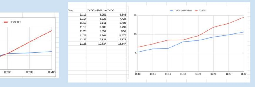
Shown in this data set is the comparison between TVOC with the lid on and off during stir frying. There is a difference of 1.193 between the two minimum values. The maximum value for boiling potato with no lid on is 14.547 while the one with lid on is 10.637.
