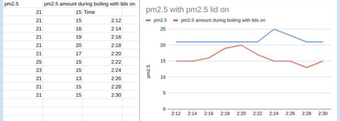
This result shows changes in PM2.5 levels over time during boiling potatoes when the wok lid was on (the bottom curve) or off (the top curve). The X-axis is the time of the day in 2-min intervals for a total of 24 min. There is a difference of six between the two minimum values and five between the maximum value
