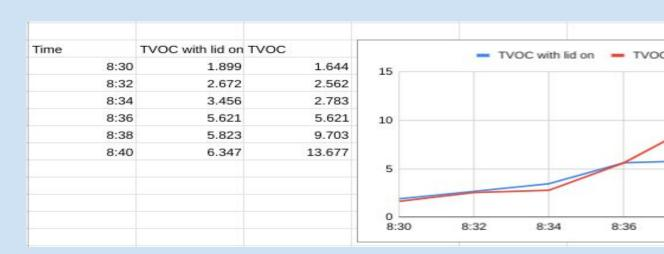
This result compare TVOC levels during frying when the lid is on (the bottom curve) or off (the top curve). There is a difference of 1.255 between the two minimum values. The maximum value for frying potato with no lid on is 13.677 while the one with lid on is 6.347.
