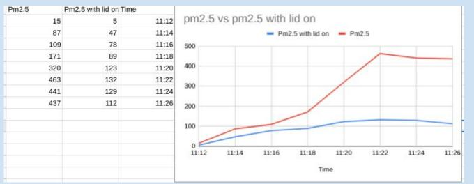
Compared here are the PM2.5 levels during stir frying when the wok lid was on (the bottom curve) or off (the top curve). As is clear, PM2.5 level was significantly higher when the lid is off (the maximum number 437) vs when the lid is on (112).
