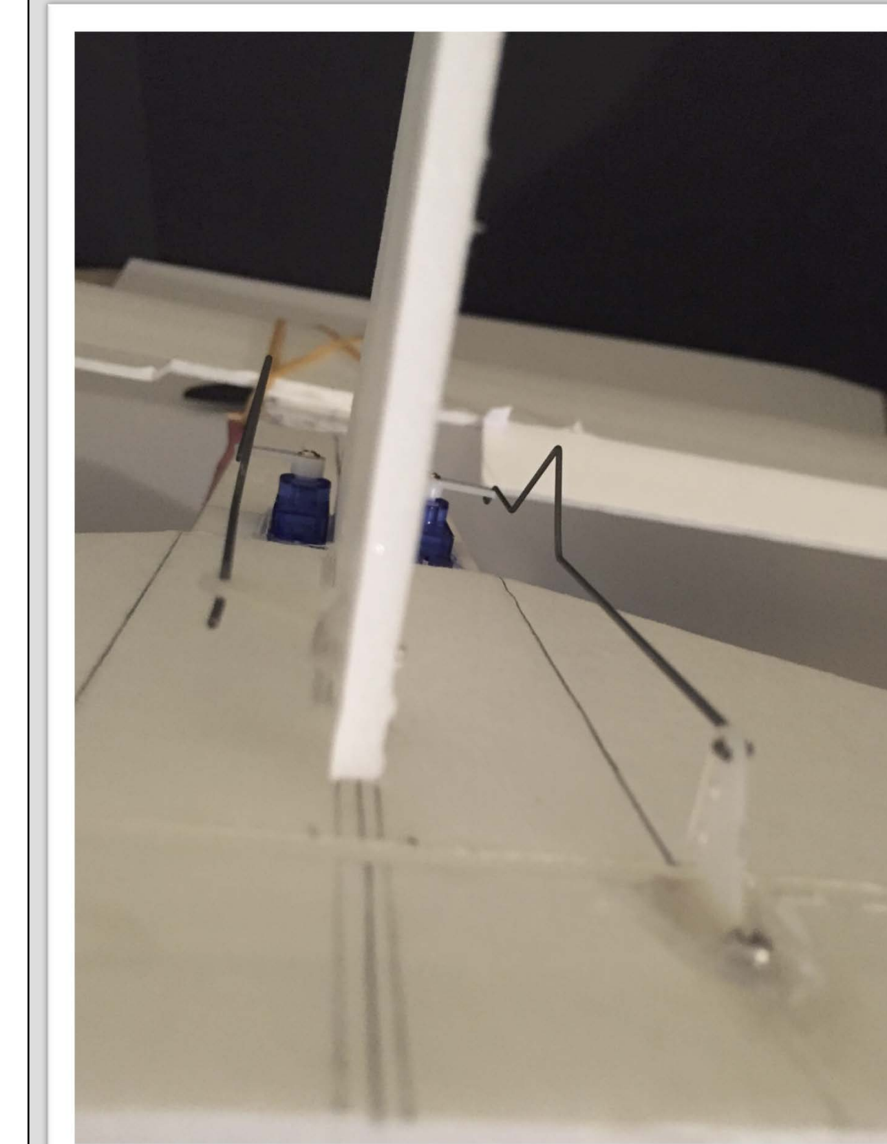
Fig. 2. Airplane tail view. Closeup of rudder and elevator servos, pushrods, and control horns.
